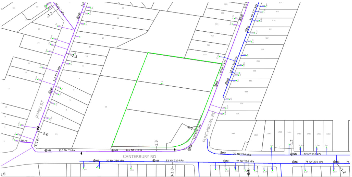
Image of gas infrastructure from Dial Before You Dig
